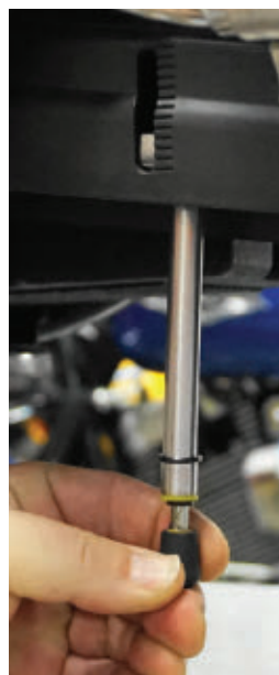
Many Harley-Davidson motorcycles have a port on the belt cover showing measurement increments, which makes adjusting belt tension easy.
