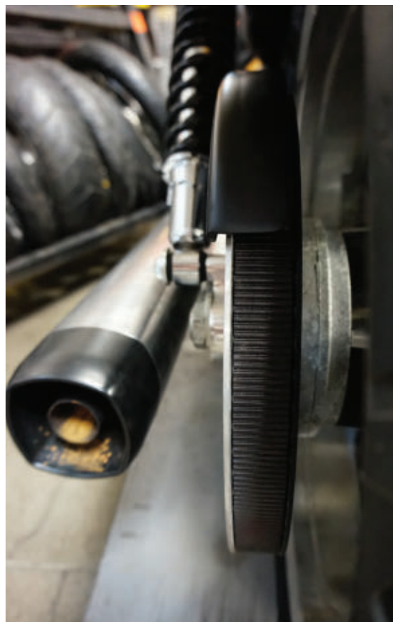
Advances in construction technology, plus their strength and light weight, have made the belts a popular choice among engineers for final drive.
