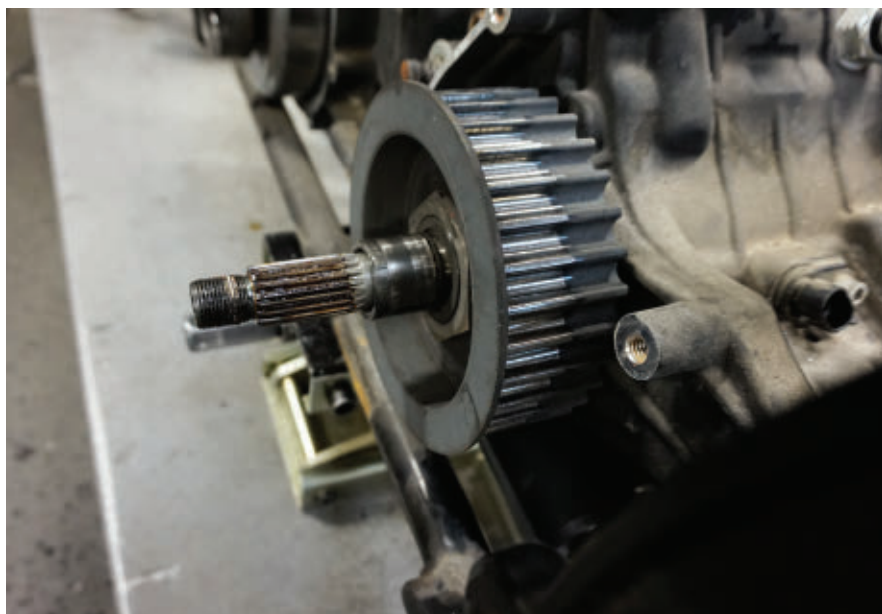
When the belt has been removed, check the sprockets for debris that may have lodged in the teeth. Replace belts that have tears along their edges.
