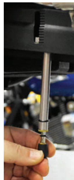
Many Harley-Davidson motorcycles have a port on the belt cover showing measurement increments, which makes adjusting belt tension easy.
